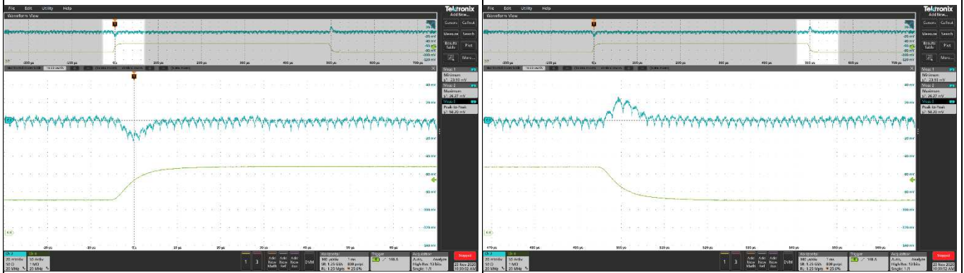
Figure 19 Transient response at 4.5 A step load current: I_o = 4.5 \text{ A} - 9 \text{ A} , (Ch2: Vo, Ch4: Io), pk-pk: 50.2 mV, fsw = 600 kHz
