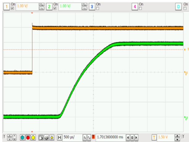
Figure 20. Turn-on Response (V CC = 3.3 V, V IN = 5.0 V, R L = 10 Ω, C L = 0.1 μF)
